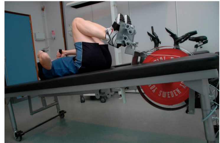
YO-YO FITNESS TRAINER, USING A FLYWHEEL TO CREATE THE FORCE AGAINST WHICH TO TRAIN
